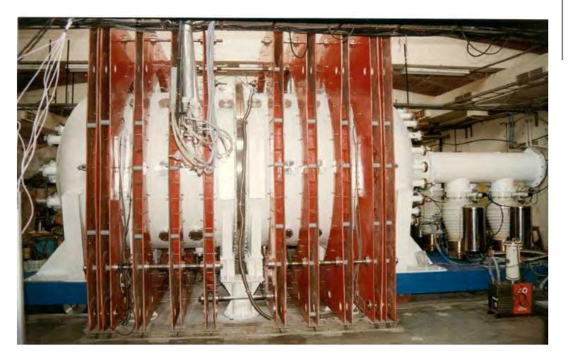
R = 2 m, L = 3 m, V = 9 m3, A = 40 m2 Double wall, Water cooled, Number of ports = 94
